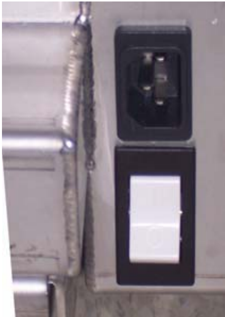
RDM Heater Power Switch
